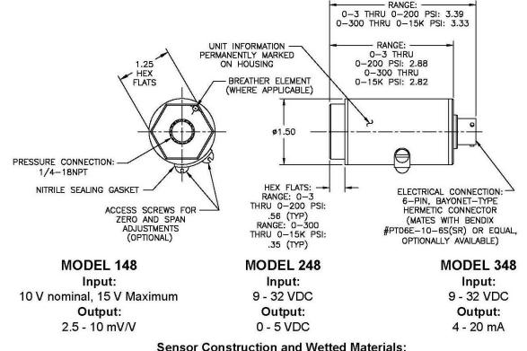
Sensor Construction and Wetted Materials: 0 - 5 thru 0 - 200 PSI: Oil Filled - Silicon - 316 Stainless Steel >200 PSI: Bonded Foil Strain Gage - 15-5 PH Stainless Steel Pressure Connection: 1/4" NPT female
