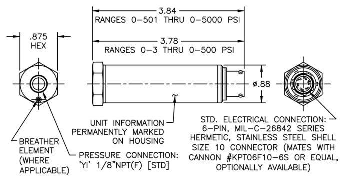
**Excitation Voltage:** 9-30 VDC; 12-30 VDC for 5 < output < -5 VDC **Output:** 0-5 VDC standard; any voltage between -10 and +10 VDC optional
