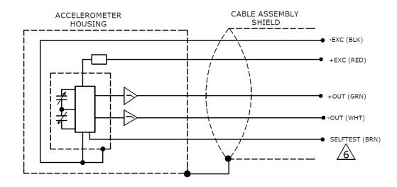
▲ BIT: CONNECT TO CIRCUIT GROUND TO PERFORM SELFTEST WHICH PRODUCES A 24Hz, 1g PEAK-TO-PEAK AMPLITUDE, SQUARE WAVE OUTPUT SIGNAL BY MECHANICALLY ACTUATING SENSOR ELEMENT. THE SELF-TEST OUTPUT SIGNAL IS IN ADDITION TO ANY INERTIAL ACCELERATION ACTING ON THE DEVICE DURING SELF-TEST. A ZERO-G ORIENTATION PROVIDES A ±0.5g SELF-TEST OUTPUT SWING AROUND ZERO-G BIAS. AN AC VOLTMETER DISPLAYS A 0.5g-rms EQUIVALENT OUTPUT SHIFT. A SINGLE-ENDED HOOKUP REDUCES THE SELF-TEST OUTPUT BY HALF.
