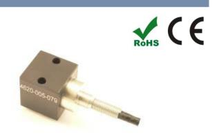
The Model 4620 is a low frequency DC response accelerometer offering outstanding performance over a wide operating temperature range. The accelerometer is available in ranges from ±2 to ±500g and incorporates a 3<sup>rd</sup> generation MEMS sensing element with integral over-range stops. The output is signal conditioned to provide a low noise amplified signal. The model 4620 incorporates a PFA insulated cable with a rugged strain relief designed for demanding applications.
