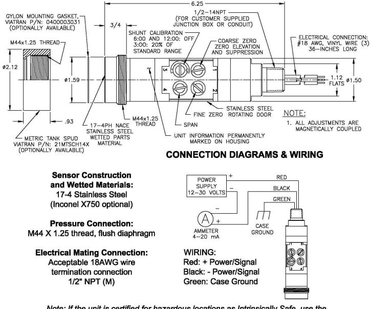
Note: If the unit is certified for hazardous locations as Intrinsically Safe, use the enclosed connection diagram. Only the pressure transmitter is considered to have the Factory Mutual safety ratings. If you have puchased a transmitter and isolator/remote seal, they have not been tested as a system for safety certification. The end-user shall be responsible for verifying the system is safe and installed accordingly.
