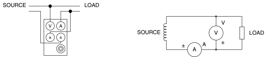
Figure 3-7 Single-Phase, Two-Wire Wiring Schematic
