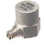
The Model 7504A is a stud mounted piezoelectric charge mode accelerometer with an operating temperature range to +260°C. The accelerometer is designed for high frequency vibration and shock measurements and offers a wide bandwidth to >10kHz and a nominal charge output of 5.6pC/g. The model 7504A features a hermetically sealed stainless steel housing and a #10-32 stud mount configuration.
