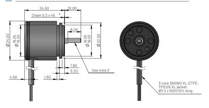
Dimensions for MHR0921 - Synchro mounting, dual output
