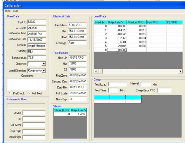
Figure 7, Sensor ID: 243738, LSB200, Calibration results performed on 11/19/2007, before vibration testing, prior to span resistance.
