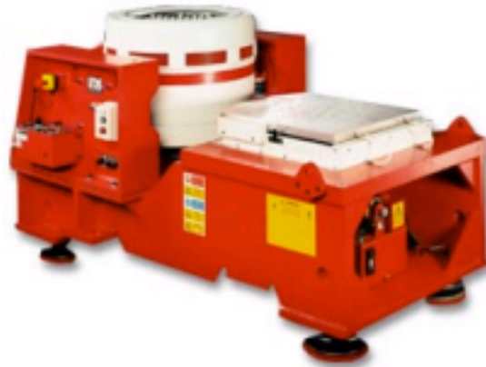
Figure 2, Low Pressure slip table, capable of vibration testing in the x, y, and z-axis.
