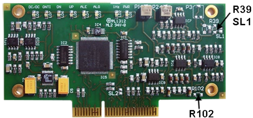
Figure 2–10 Location of resistors R102, R39; SolderLink SL1 the DES 410 & DES 411 circuit
