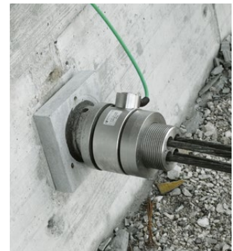
Fig. 2: HRL 4 (4 strands) mounted on cable anchor
