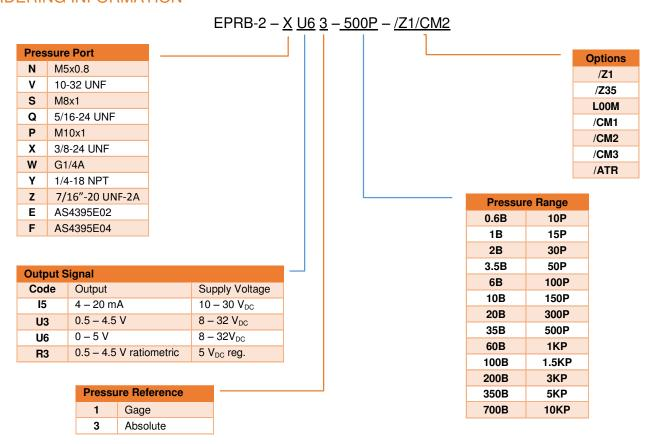
The **psi** range models are only supplied with imperial thread design. The **bar** range models are only supplied with metric thread design.
