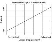
**Output Characteristic:** Target position at start of normal travel is 36.0 mm from seal face. The output increases as the target is moved away from the sensor body, the calibrated stroke is between 5 mm and 800 mm.
