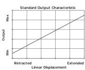
**Output Characteristic:** Target is extended 7 mm from end of body at start of normal travel. The output increases as the target extends from the sensor body, the calibrated stroke is between 5 mm and 800 mm.
