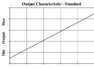
Retracted Linear Displacement Extended
