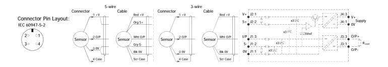
Approval only applies to specified ambient temperature range and atmospheric conditions in the range: 0.80 to 1.10 Bar, oxygen  $\leq$  21%. The H100 is available with the following connections:-
