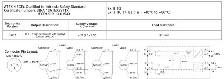
Putting Into Service: The sensor must be used with a galvanic isolation barrier designed to supply the sensor with a nominal 5V and to transmit the sensor output to a safe area. The barrier parameters must not exceed:-
