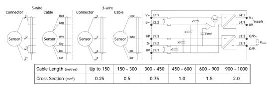
The table above shows recommended conductor sizes with respect to cable length for both three and five wire connections, based on copper conductors. Three wire connections will introduce a gain reduction of 5% and a ±1% temperature dependence of gain over the range -40°C to +80°C for the cable temperature. (i.e. about -150 ppm/°C for the maximum lengths shown and less pro rata for shorter lengths.)
