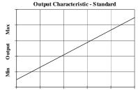
Retracted Linear Displacement Extended
