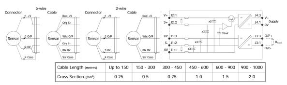
The table above shows recommended conductor sizes with respect to cable length for both three and five wire connections, based on copper conductors. Three wire connections will introduce a gain reduction of 5% and a ±1% temperature dependence of gain over the range -40°C to +80°C for the cable temperature. (i.e. about -150 ppm/°C for the maximum lengths shown and less pro rata for shorter lengths.)
