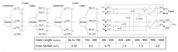
The table above shows recommended conductor sizes with respect to cable length for both three and five wire connections, based on copper conductors. Three wire connections will introduce a gain reduction of 5% and a ±1% temperature dependence of gain over the range -40°C to +80°C for the cable temperature. (i.e. about -150 ppm/°C for the maximum lengths shown and less pro rata for shorter lengths.)
