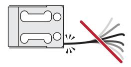
3. Properly secure sensor cable to limit cable movement influence.
