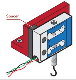
3. Additional Pin holes are available to help with support on the higher capacity 200lb LSM300.
