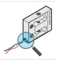
2. Avoid stress and movement on cable to avoid damage.
