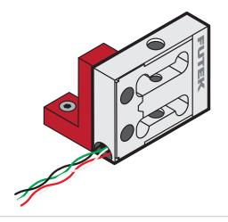
2. Deflecting surfaces must be free from contact or interference. Spacers may be used to help isolate sensor from surfaces.
