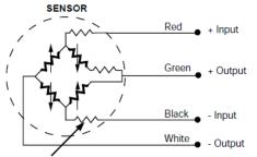
Compensation resistors in external module on some models
