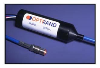
The AutoPSI-TC - temperature compensated dynamic pressure sensor is uniquely capable of long term operation in high temperature up to 360°C, at high levels of Electromagnetic and Radio Frequency (EMI/RFI) fields, and in chemically volatile media.
