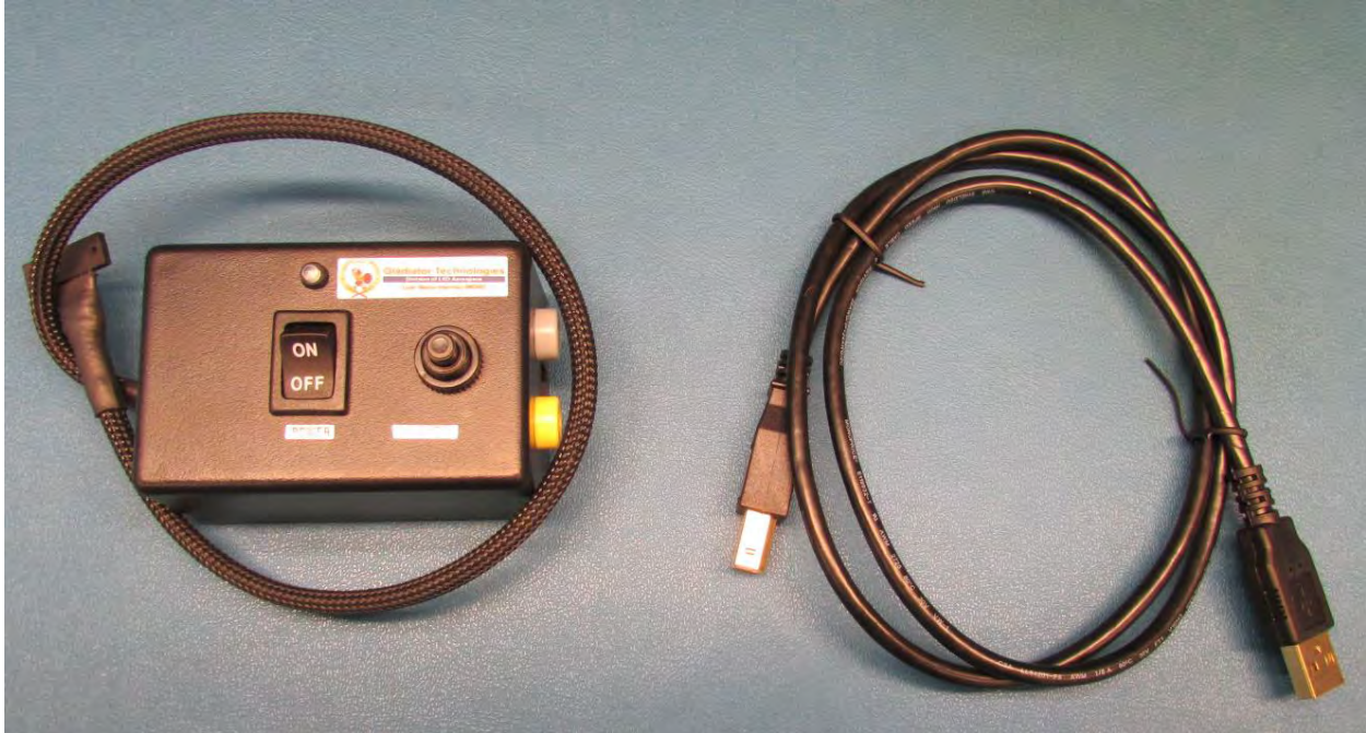
Figure 1 SDK Power Control/Self-Test, SDK to PC Cabling
