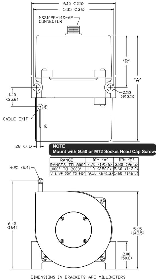
DIMENSIONS IN BRACKETS ARE MILLIMETERS
