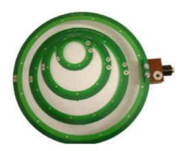
The IL2 features a set of glass-fibre loops which form the stationary part of an inductive power and signal pickup system. If the physical situation permits, they are the preferred technique giving the maximum power transfer, especially for multi-channel systems. Customised single turn copper loops can easily be fabricated to replace the fibre-glass loops. The copper loops could, for example, be oval to accept greater shaft displacement in one axis.
