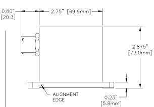
NOTE: IN ADDITION TO THE ALIGNMENT EDGE SHOWN, THE THREE MOUNTING FEET CONSTRUCT AN ALIGNMENT PLANE. WHILE FASTENING THE UNIT, PRESS THE ALIGNMENT EDGE SECURELY AGAINST THE ALIGNMENT RIDGE.
