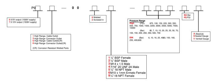
Examples : P90600027K5PSS = 0 to 5V output from 10 to 36V supply, cable outlet, welded ¼" BSP male port, 7500 psi sealed gauge
