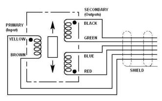
Connect Blue and Green wires together for differential output
