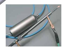
The PSIglow™ integrates Optrand's miniature 1.7mm diameter, fiber optic sensor with a fully functional ceramic heater-based glow plug allowing cylinder pressure monitoring of diesel engines without head modification or loss of glow plug functionality.
