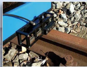
None contact web/base of the rail measurement
