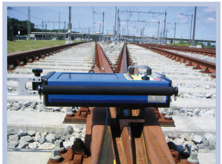
Fig. 4: Turnout Measurement with Railmonitor
