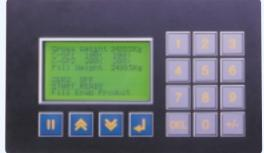
The combination of a Tracker 240 and an HMI, fitted with a Modbus compatible RS485 interface, becomes a powerful stand-alone batch control system and recipe selection system. The HMI's display and function buttons can be tailored for any application and language. Many HMI units can also be a gateway for Fieldbus connection (e.g. Profibus, Device Net). A single HMI can communicate with up to 32 Tracker 240 units.
