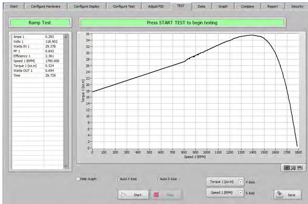
Figure 9–3 Ramp Test Screen
