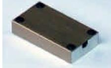
In construction the transmitter circuitry is encapsulated in epoxy-resin within a rectangular housing precision machined from aluminium. Isolation from the inductive power supply and other interference source is provided by a close fitting metal screening fabricated in high-permeability metal. A slotted baseplate simplifies attachment using the CAK kit steel strapping.
